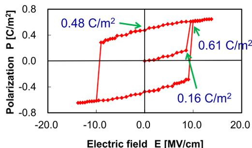
FIG. 2. Calculated  $P$ - $E$  hysteresis loop for  $\text{AgNbO}_3$ .
