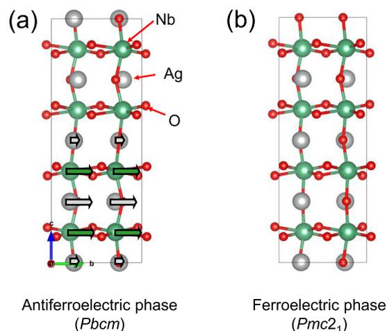
FIG. 1. Crystal structures of  $\text{AgNbO}_3$ : (a) antiferroelectric  $Pbcm$  phase and (b) ferroelectric  $Pmc2_1$  phase. The atomic displacements under an electric field are shown in panel (a). Displacement of the ions under a finite electric field reduces the symmetry from  $Pbcm$  to  $Pmc2_1$ . Loss of centrosymmetry in the  $Pmc2_1$  phase causes  $\text{AgNbO}_3$  to become ferroelectric.
