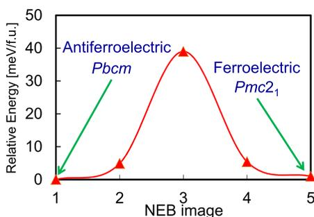
FIG. 3. Potential surface within  $AgNbO_3$  during the ferroelectric phase transition from  $Pbcm$  to  $Pmc2_1$  under a finite electric field.
